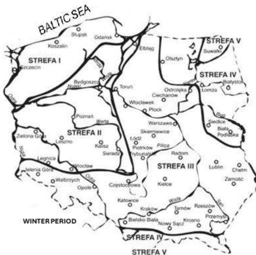
Fig. 1. Division of Poland's area into climate zones depending on the calculation of the external temperature to be used in determining the heat demand for space heating
