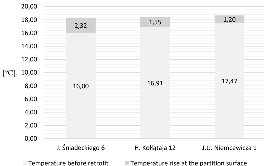
Fig. 9. Increase in the design temperature on the internal surface of the envelope resulting from the insulation of curtain walls in the buildings included in the analysis
